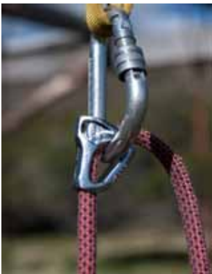
1. Progress capture with a Tribloc
