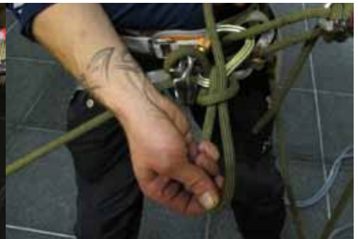
3. Pass a loop through that loop, and pull towards the belay plate.
