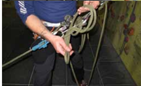
3. Pull the loop out to make a long tail, and then tie off the hitch with two half hitches around the live rope.
